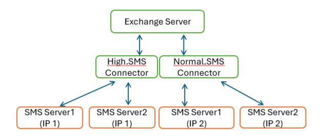
Each SMS Server has 2 x IP addresses assigned to a single VNIC.
